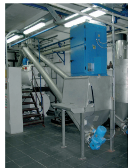
Bag deposit system with filter unit and dosing screw.
