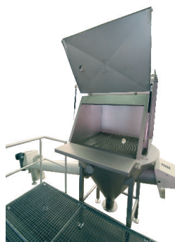
Bag deposit system fed by dosing screw.
