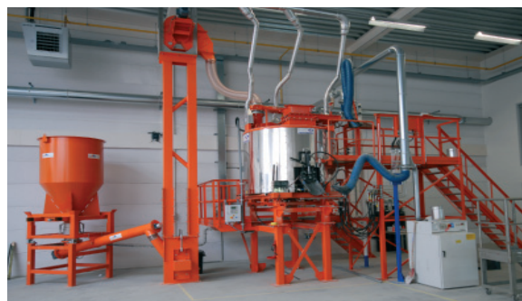
Laboratory set-up for the production of sulphur concrete. Weighed dosing screw brings sulphur pellets to the elevator, which conveys them vertically.
