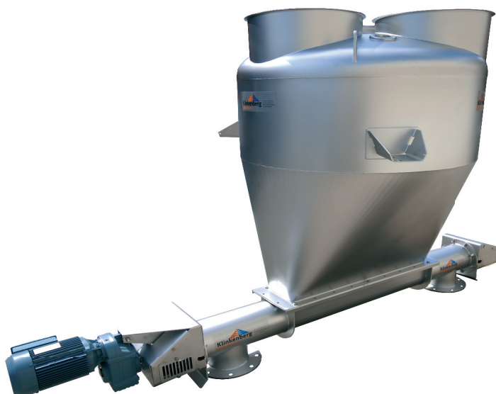
1500-litre hopper with dosing screw measuring out to right or left
