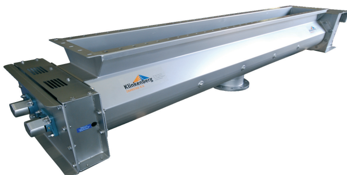
Double-shaft paddle mixer with breaker pins for breaking agglomerates that are produced during the mixing of sticky products.
