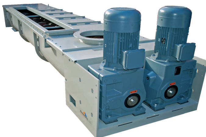
Double-shaft paddle mixer for mixing fly ash slurry with dried fly ash. The shafts are powered separately. Paddles are made of hardened steel and welded on with Vautid 100. Average hardness 750 to 1000 HV
