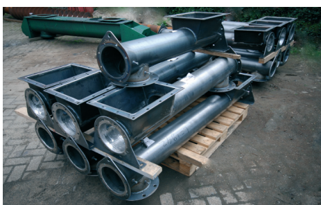
Production of steel tube conveyor jackets.
