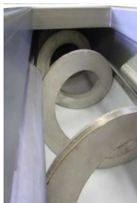
Shaftless screw conveyor entirely constructed from stainless steel 316L, equipped with hold-down bars
